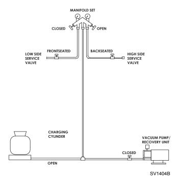
Figure 7-8. Charging Connections
